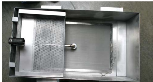
Remove the crumb screen by lifting it up and out.
